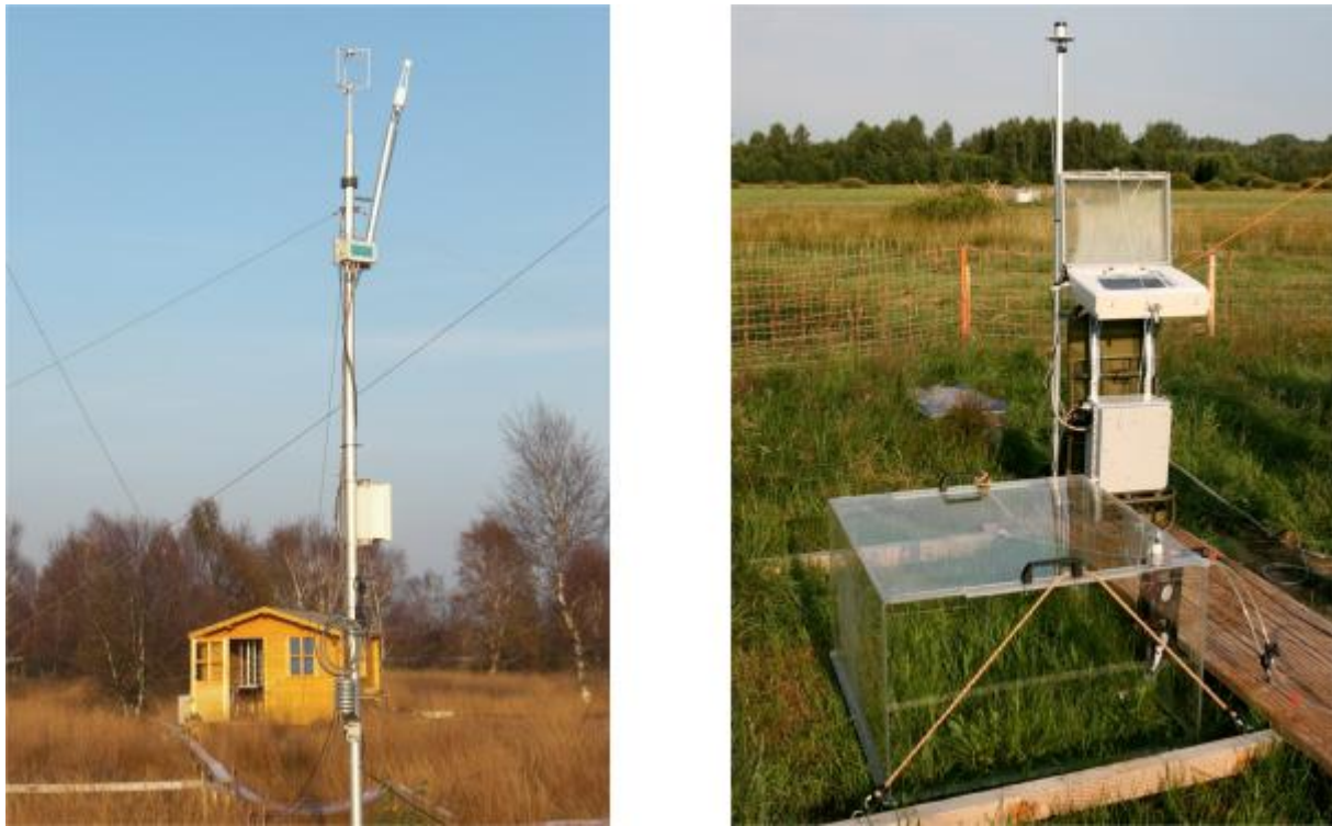
Figure 1 – Eddy covariance tower (left) at a semi-natural peatland [10] and a transparent chamber connected to a portable analyzer for the measurement of NEE at a grassland site [12].
