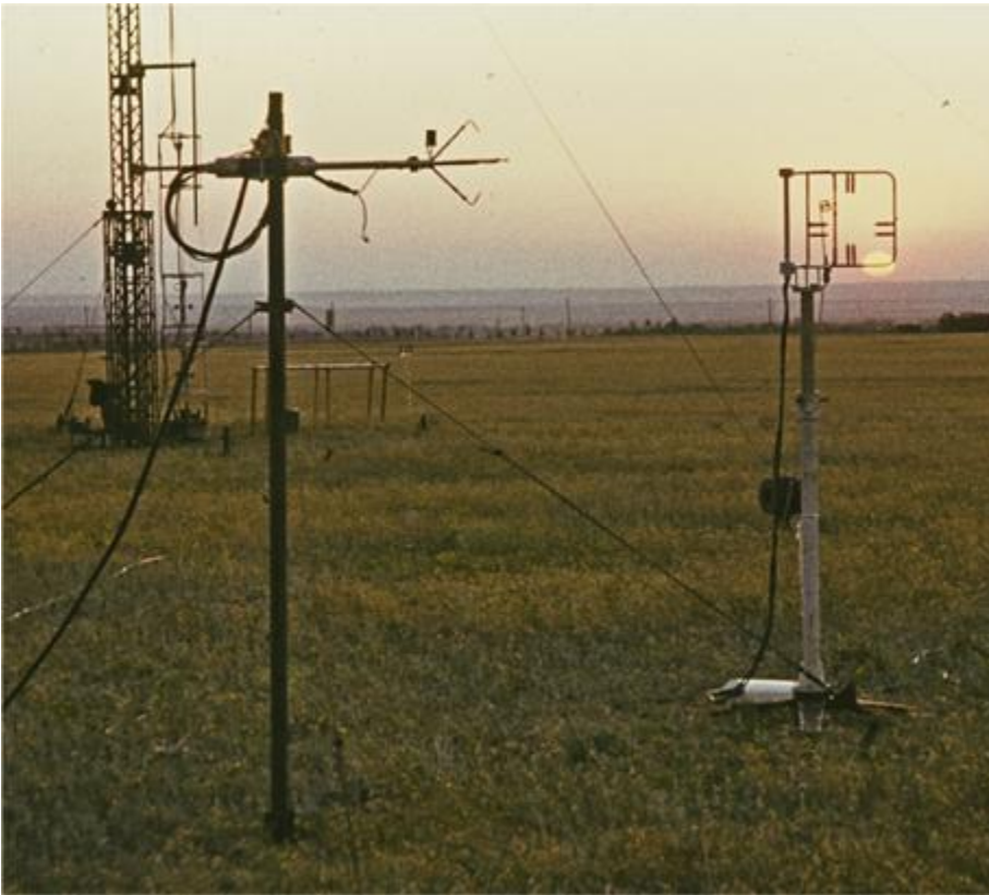
Figure 1 – Russian phase shift anemometer during the experiment ITCE-81 [6] at the Tsymlyansk research area (left) together with the Japanese Kaijo-Denki sonic anemometer PAT 300, working with the travel time principle (Photograph: Foken)
