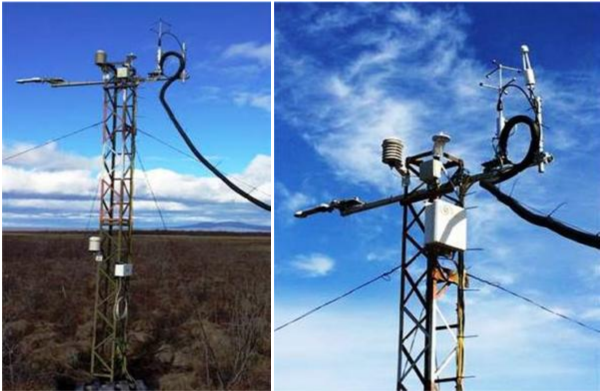
Figure 3 – Eddy-covariance towers at the Chersky research site (Photograph: Göckede). The system consists of a heated sonic anemometer (METEK USA1), an open-path gas analyzer for CO 2 /H 2 O (LiCor 7500, only right picture), and the inlet line for a closed-path gas analyzer for CH 4 /CO 2 /H 2 O (Los Gatos FGGA).
